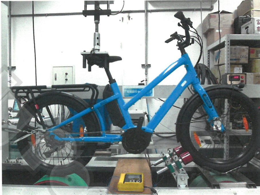
Fig. 5-1 Electric cables and connections discharging temperatures test.
